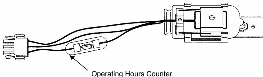
**Figure 22 Pre-aligned Deuterium Lamp Assembly (B0160917)**
