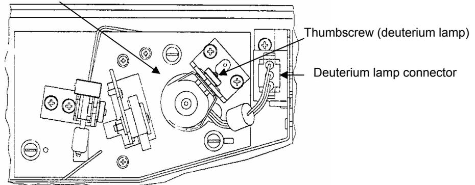
**Figure 23 Removing the deuterium lamp connector**
