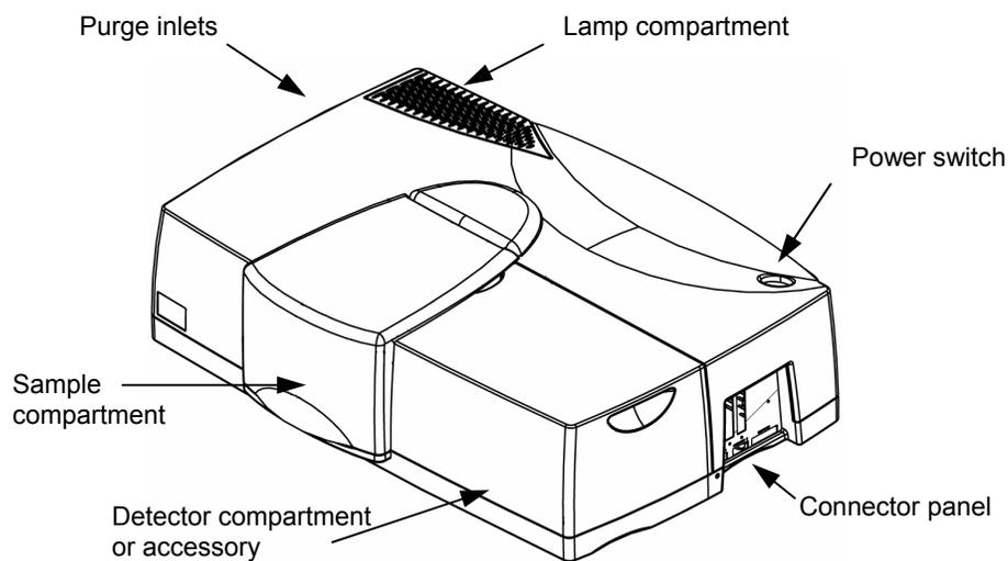
**Figure 6 Lambda 650/850/950 spectrometer features**
