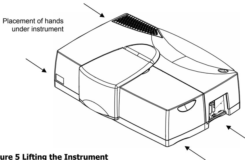
**Figure 5 Lifting the Instrument**
