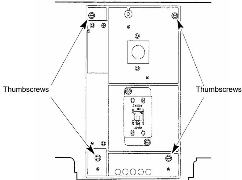
**Figure 24 Four thumbscrews on the sample compartment baseplate**
