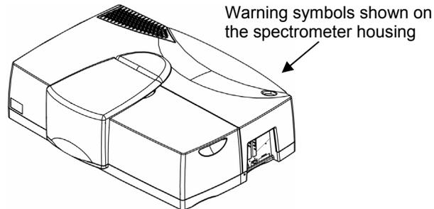
Figure 1 Lambda 650/850/950 Spectrometer
