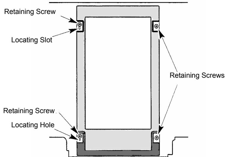
**Figure 25 Four retaining screws in the sample compartment**
