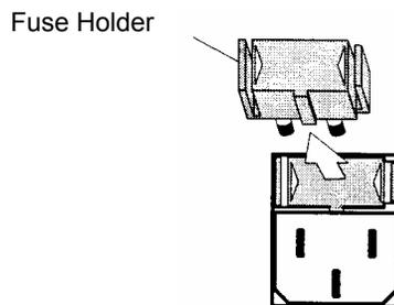
**Figure 4 Removing the fuse holder**
