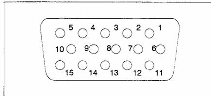
**Figure 31 Pin configuration of 15-pin connector**
