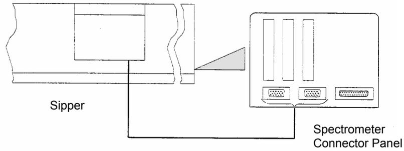
**Figure 30 Sipper, electrical connection**
