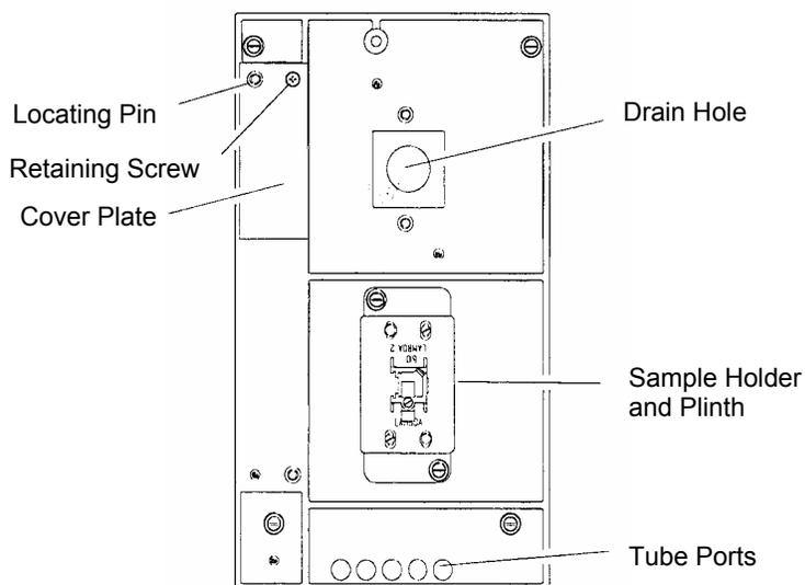
**Figure 14 Lambda 650/850/950 Sample Compartment Baseplate**
