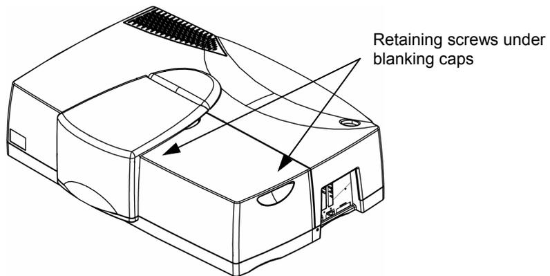
**Figure 26 Undoing the retaining screws**
